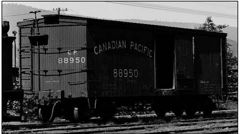
The Canadian Pacific preferred two trussrods on their cars ends, and built nearly 25,000 cars with them. DL&W company photo, Steamtown NPS collection.
