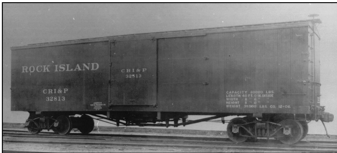
With its seasonal grain traffic in mind, the Rock Island transitioned to 40-foot long boxcars before most other railroads. Understanding bowing stresses better than some other roads, the Rock added their end trussrods low on the car ends. Al Westerfield collection.
