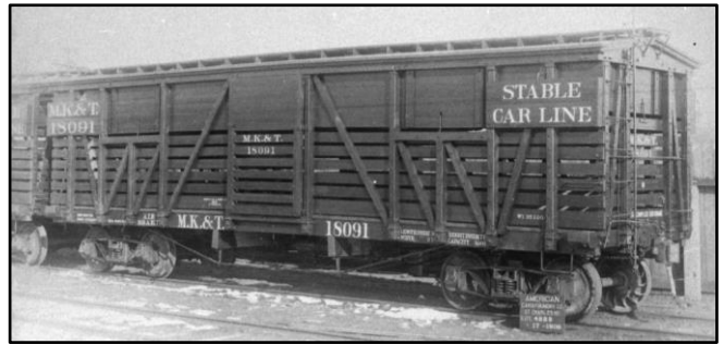
The Katy had a real love affair with trussrod ends. Starting in the early 1890s and extending to 1916, the railroad added them to every car they could, including ventilated boxcars, stock cars, and even gondolas! All photos Al Westerfield collection.
