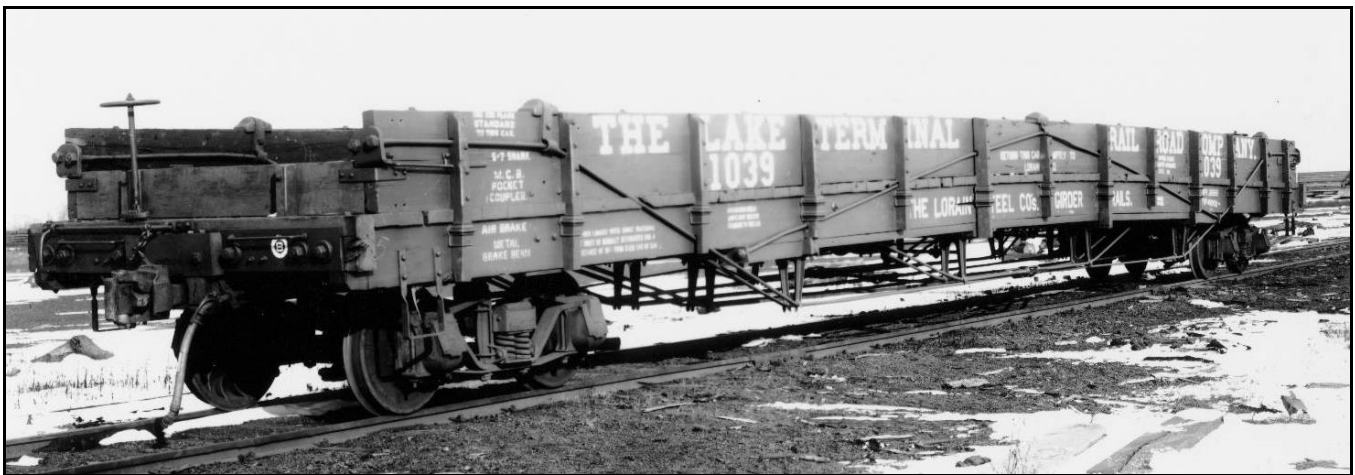
Probably the most extreme examples of trussed up gondolas were the 100 cars of the Lake Terminal Railroad's 1000-2000 series. These 63-foot long, "all wood" cars were designed to move long dimensional steel loads from the mills of Lorain, Ohio. Author's collection.
