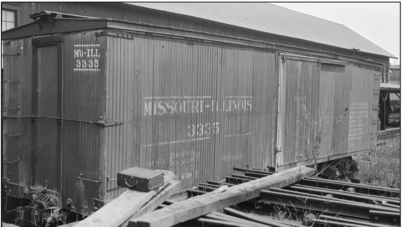
M-IL 3335 has a 4/1929 reweigh date, and still has its original end trussrods in this Depression era photo. Author's collection.
