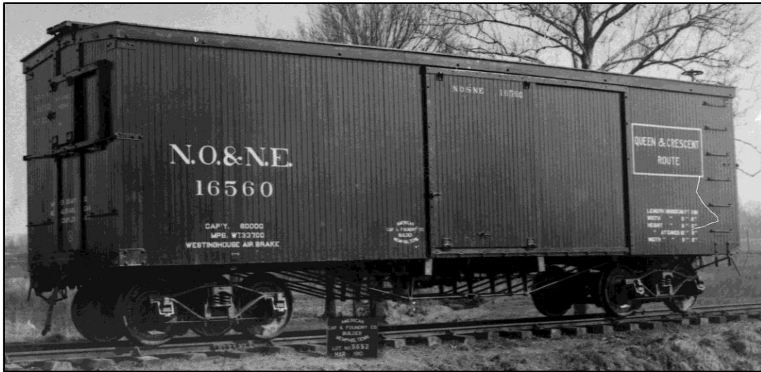
By 1910 car designers knew that steel needed to be added to car ends, but some railroads continued to build cars with wood ends and trussrods, hoping that they'd be strong enough. NO&NE 16560, an ACF Memphis product from 1910, shows one such later-built car. ACF photo, Al Westerfield collection.
