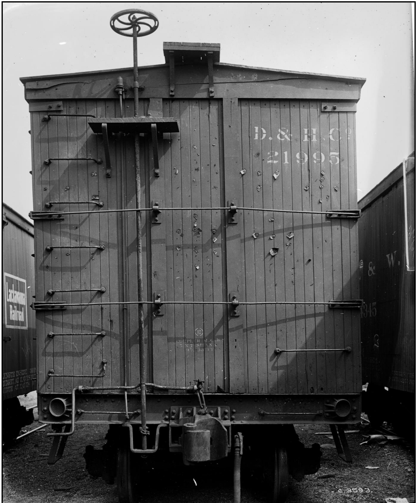
Most of the D&H's house cars, including box, auto, stock, and refrigerator cars, were built with trussrodded ends between 1905-1907. This image of D&H 21995 is a wonderful study of how these rods were added to cars. DL&W company photo, Steamtown NPS collection.
