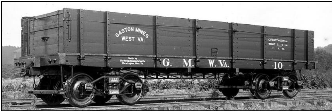
An interesting footnote to the idea of strengthening a freight car with trussrods were the few gondolas built with trussrods on their sides, in an attempt to keep them from excessively bowing outward during harsh treatment at mines. Never very popular, by 1900 the idea had been dropped in favor of all-steel gondolas. Both photos J.W. Barriger photo, St. Louis Mercantile Library collection.
