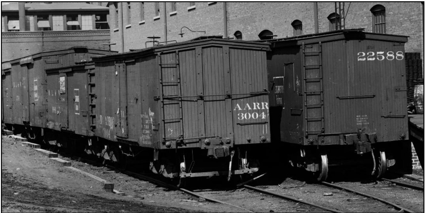
AA 3004 is seen here with trussrodded ends, while DL&W next to it does not. In theory the Ann Arbor car has “stronger” ends, but in practice that wasn’t the case. DL&W company photo, Steamtown NPS collection.
