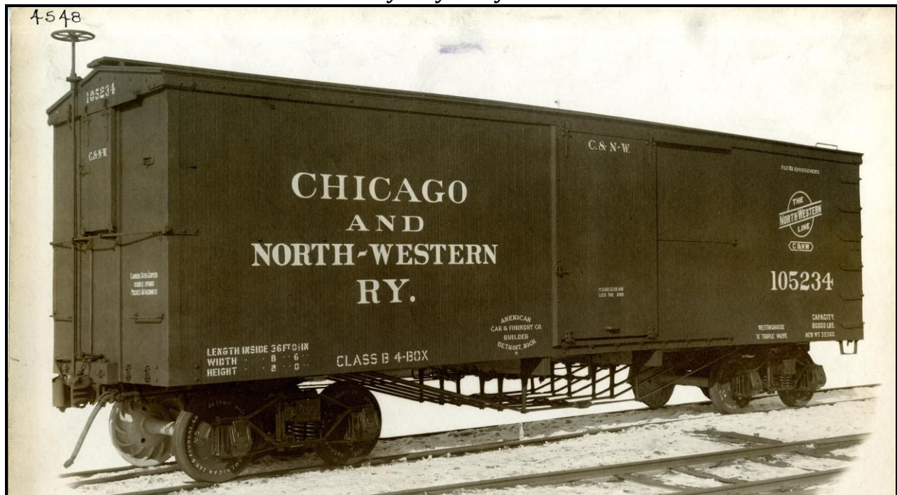
C&NW 105234, built at ACF's Detroit plant in early 1907. The end trussrods and their corner braces were an early attempt to strengthen house car ends. Barriger Library collection.
