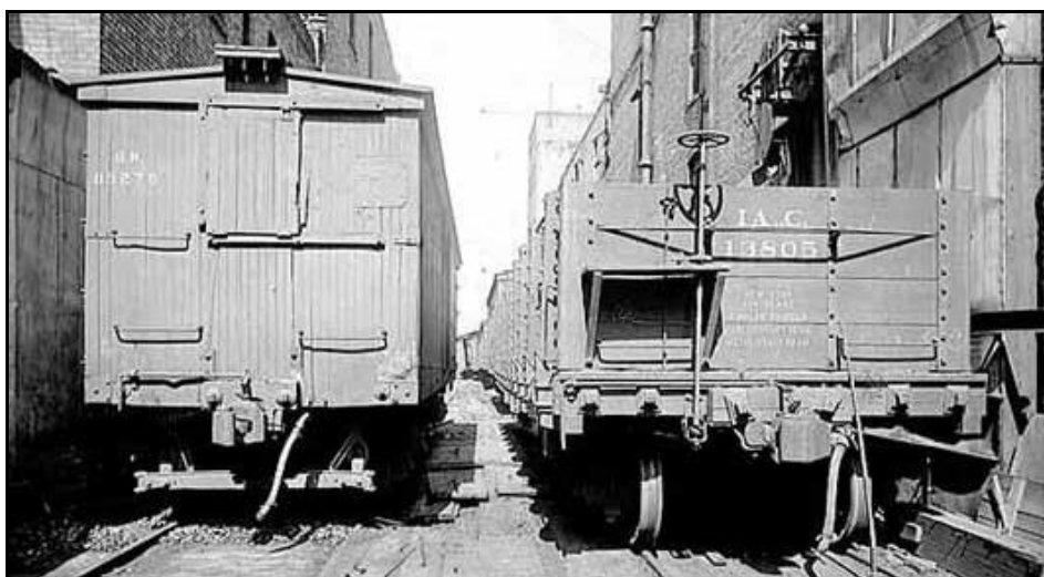
Oddly, there were even a few gondolas built with trussrod ends. Iowa Central 13805 was one of 250 such cars, built around 1905. These cars eventually went to the M&StL, and were quickly scrapped. Author's collection.
