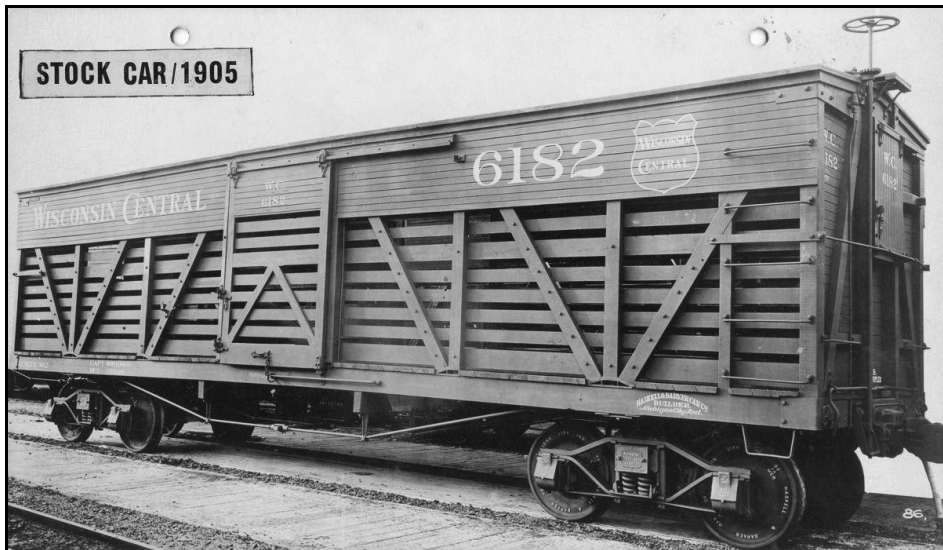
Stock cars with trussrod ends were far more common than reefers. WC 6182 was built in 1905 by Haskell & Barker. Author's collection.
