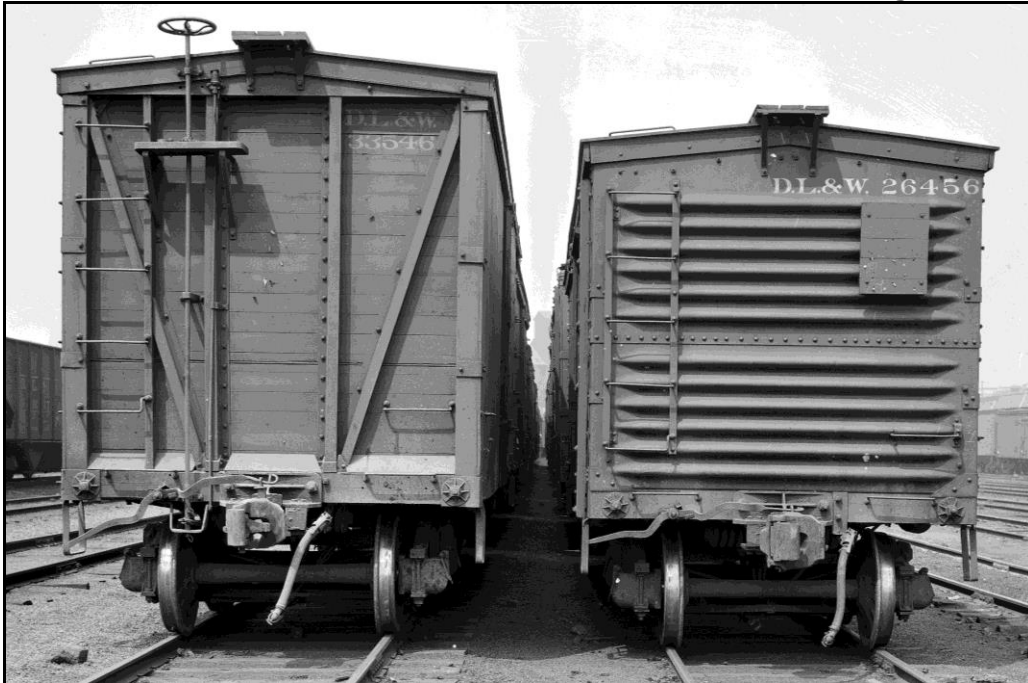
Two DL&W boxcars show off two different steel ends, both of which were far more successful than trussrods. To the left is a car with “Indestructible” ends, and to the right is a car with corrugated, all-steel ends. DL&W company photo, Steamtown NPS collection.
