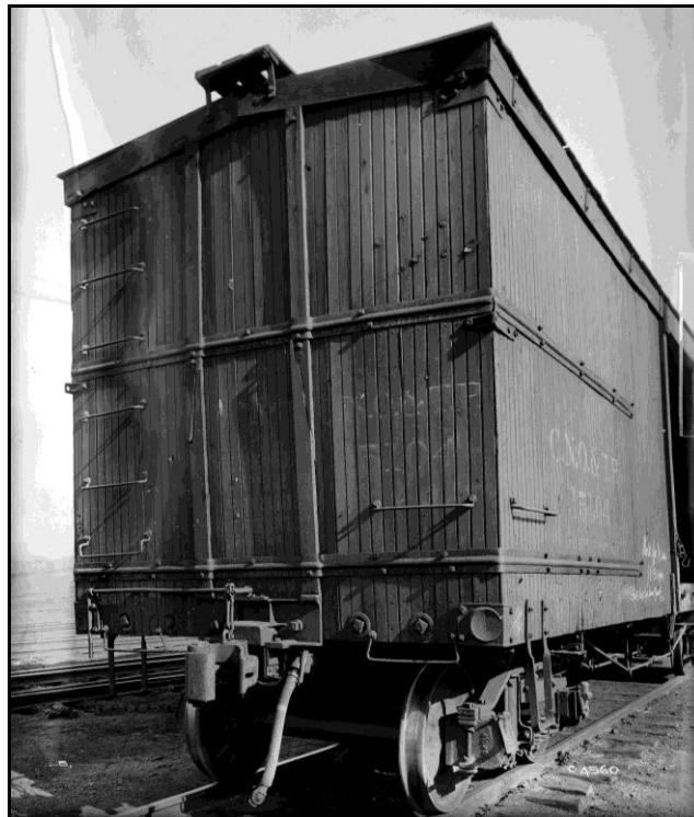
When trussrods failed to strengthen car ends, some railroads experimented with other methods to shore up boxcar ends, without resorting to the cost of a full steel end. CNO&TP 15104, seen in Newark NJ in 1918, has custom formed, hat section ribs added, in an attempt to do what the trussrods couldn't. The side legs of these ribs extend almost six feet along the car sides, and even they couldn't take crash stresses: the ribs are cracked at the corner. And both end beams are cracked. DL&W company photo, Steamtown NPS collection.
