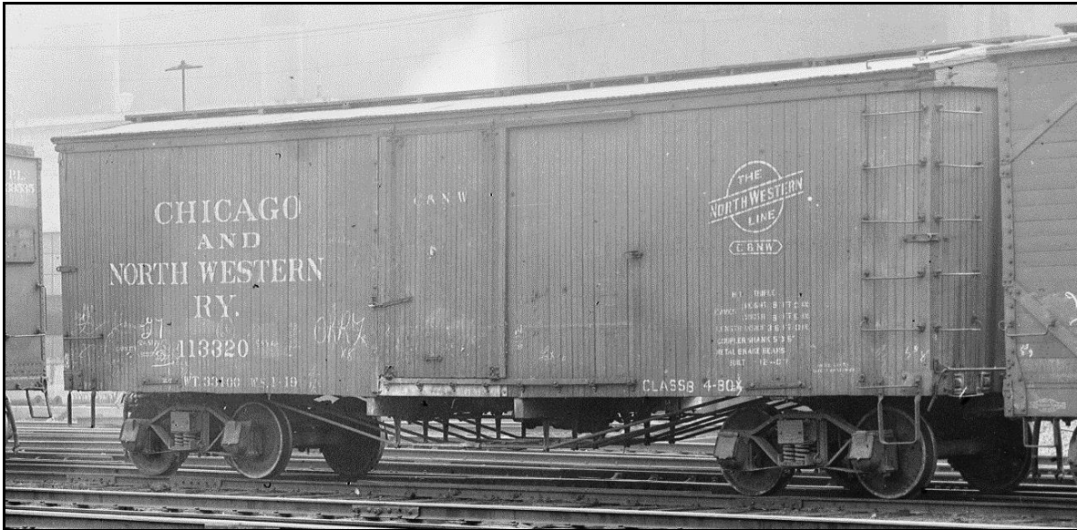
By WWI railroads were quickly realizing that trussrods on the ends of boxcars weren't worth the effort, and began removing them. C&NW 113320, seen in Hoboken NJ in 1919, is one such car. The corner braces remain, but the rods are gone. DL&W company photo, Steamtown NPS collection.
